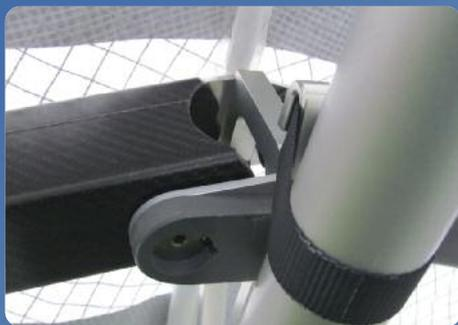
The top of the A-frame has been cleverly fully enclosed, minimising drag in the last "open" area left on a typical flexwing. The VG pulley block has been re-routed and is much lighter to use. The VG cleat design has been changed too and is much better than the 150 one. The cleat works in reverse to most cleats (pull back to lock) and takes a little getting used to, but overall it is a very ergonomic solution.
